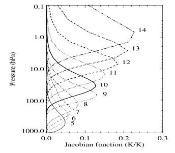
**Figure 1**: AMSU-A weighting functions on the 43 RTTOV levels computed using the US standard atmosphere. Each function is identified by a channel number on the right. Only weighting functions for channels 5 to 14 are shown. Figure courtesy of D. Shawn Turner.
